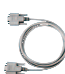
RS-232C CABLE 9637 For the PC, 9 pins - 9 pins, cross, 1.8m (5.91 ft) length
